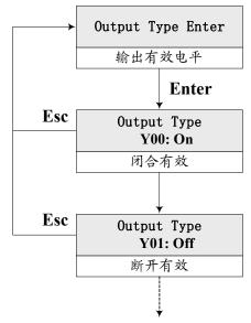
▲ Note: When the output relay Y12 uses Fuji frequency inverter, the able signal should be set OFF.
