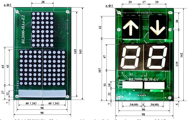
Diagram 3-3-4-6 BL2000-HAx-E2 Appearance and layout installation dimension Diagram 3-3-4-7 BL2000-HCH-G1 Appearance and layout installation dimension
