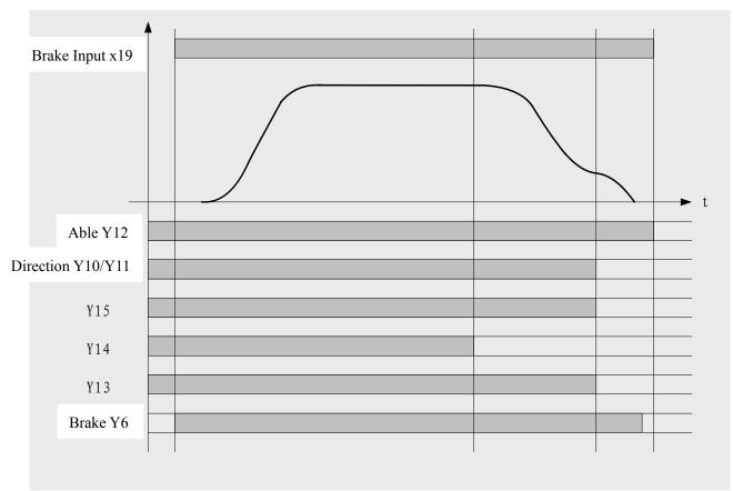
Table 5-6-2-6 (8)The sequential diagram of main control boar output when FU12<br/>and FU13 are set on
