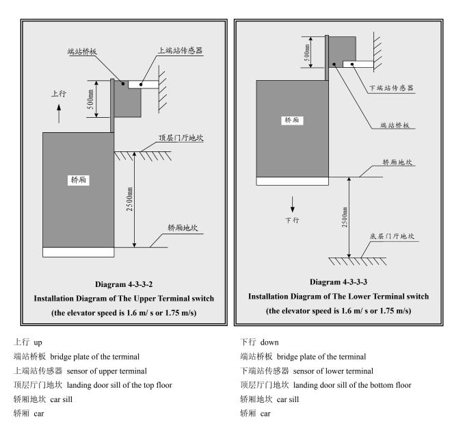
The installation position of the terminal when the multi speeds are given has something to do with the setting of the speed changing distance of the segment speed:
