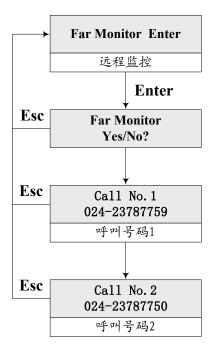
The calling number can only be set if the function of remote monitoring is set **Yes**. If there is something wrong with the elevator, the system will automatically call the set telephone number. Remote monitoring could call two telephone numbers to the maximum.
