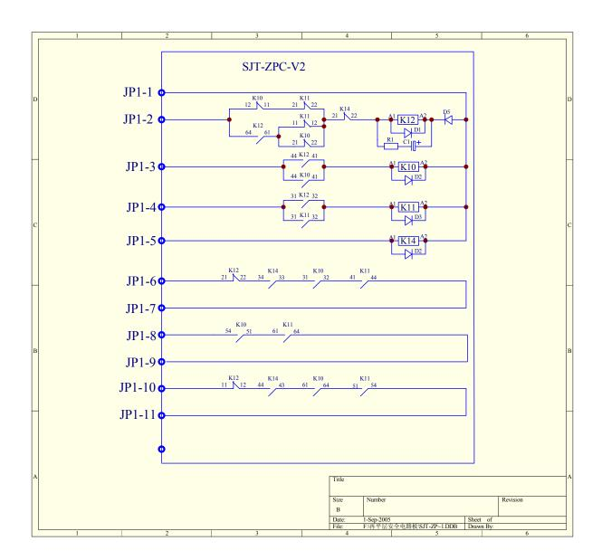
1. Safety Circuit Board (SJT-ZPC-V2) Schematic Diagram
