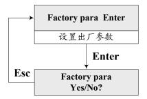
Select Yes and the parameters will be restored to the factory parameters. When the system debugging parameter setting is disordered and needed to be reset, this function should be applied.
