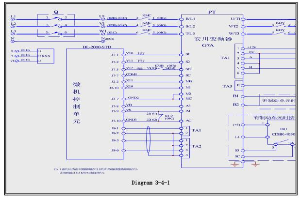
1. BL2000 Serial Control System - Frequency Variable Adjusting Speed Loop Schematic Diagram
