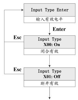
Table 5-4-2-The setting of effective electrical level at the input port
