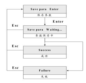
▲ Note: the parameter which could be set will take effect instantly after modification. But if the parameter is not saved after modification, after turning off the power supply of the system, the parameter will be restored to the original one.
