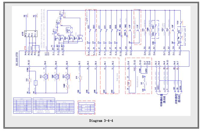
呼梯/操纵盘通讯线 并联/群控通讯线 Call/control panel phone communication wire Parallel/group communication wire
