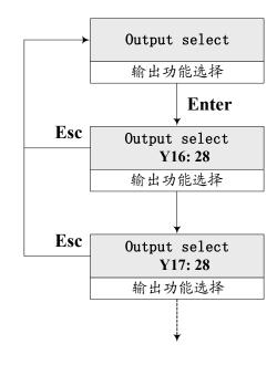
Output ports Y16 and Y17 of new main board BL2000-STB-V9 are multifunctional output ports. Set as corresponding function numbers, Y16 and Y17 will output the corresponding functional signals.
