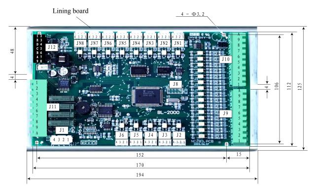
Diagram 3-3-2-1 Appearance and layout installation dimension of car board BL2000-CZB
