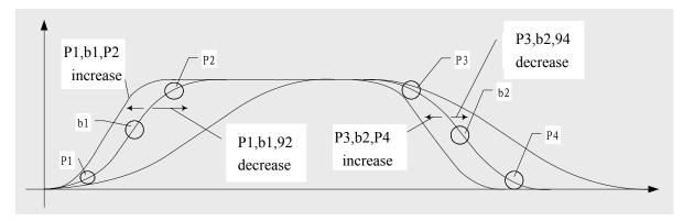
Table 5-5-1-9 The diagram of speed curve parameter adjustment
