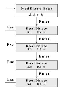
In the multi speed modes, regulating the decelerating distance of multi speeds could prevent the elevator from braking at non zero speed or overlong creeping distance. The decelerating distances which correspond to different speeds are different, which are need to be tested and set when debugging. Only take the table 5-6-2-1 in (10) as reference information when setting the parameters.
