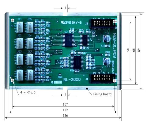
Diagram 3-3-3-1 Appearance and layout installation dimension of car expansion board BL2000-CEB 1. Instruction
