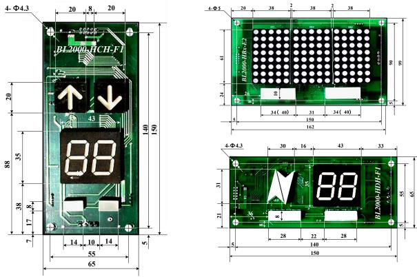
Diagram 3-3-4-8 BL2000-HCH-F1 Appearance and layout installation dimension Diagram 3-3-4-9 and 10 BL2000-HBx-E2, HDH-F1 Appearance and layout installation dimension
