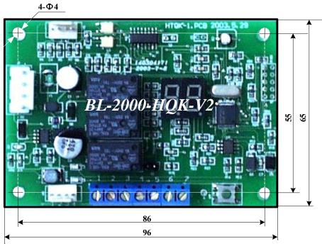
Diagram 3-3-5 Appearance and layout installation dimension of group control and call boardBL-2000-HQK
