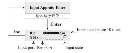
The heights of bars represent input port logic levels. High: 1, low: 0. If the quantity of 1 of input port in the bar chart is closer to that of 0, the interference is more intense.
